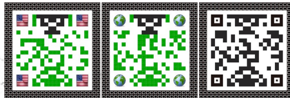
Fig-7: GCODE-18-Bytes-UTF-8: [Data+3x:Border] with Max of [24x24] Dot-Matrix
