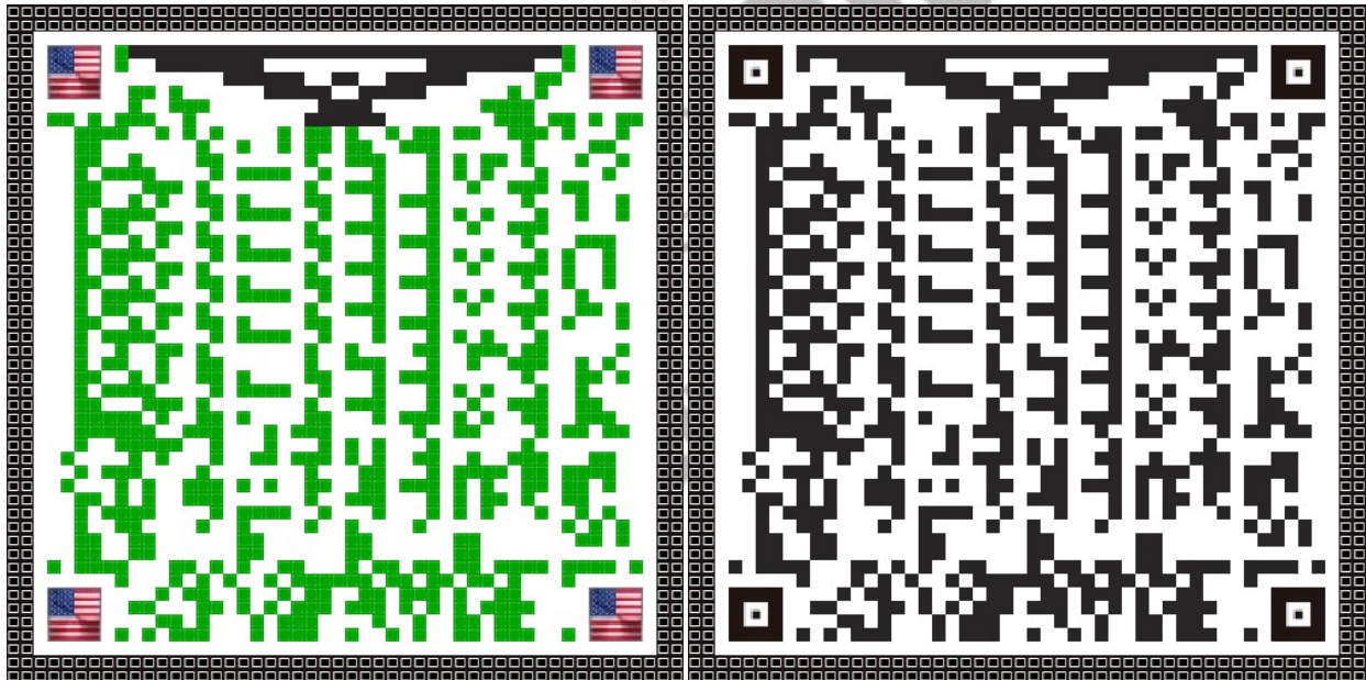
Fig-14: GCODE-Label: [32x32:Data]+[50x50 (6x:LineChecksum+3x:Border)]
